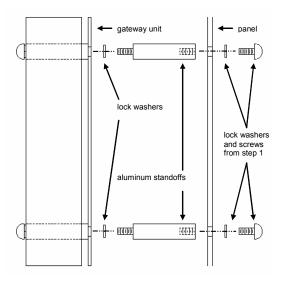
Figure 1: Standoff Kit Installation
